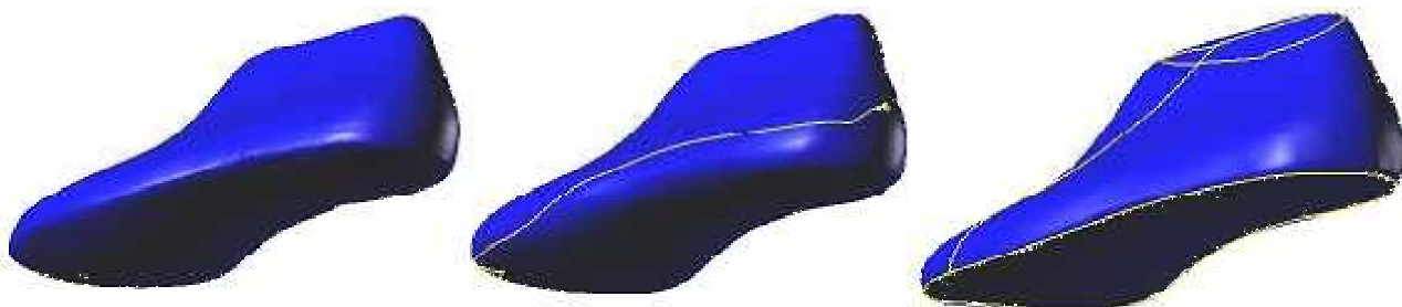
Fig.3.From Left to Right: Mesh, Single Surface, Three Surface Last
