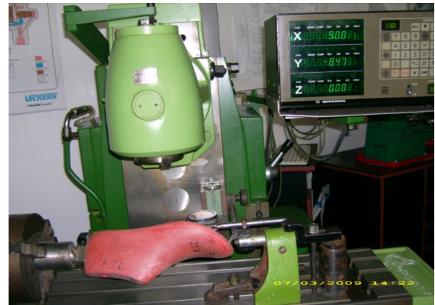
Fig.7. How is positioned the shoe last in CNC milling machine
